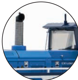
Exhaust pipe panelling made from photo-etched
